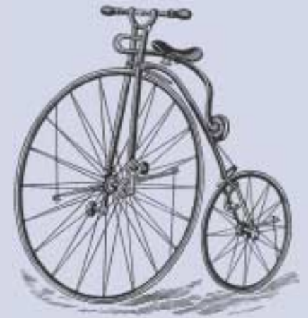
The first wheel built with tensioned wire spokes was the Ariel built by James Starley in 1870.
